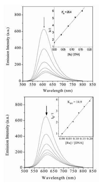
**Figure 3.** Emission spectra of complexes **1** (top) and **2** (bottom) in Tris–HCl buffer in the absence and presence of CT–DNA. Arrow shows the intensity change on increasing DNA concentrations.
